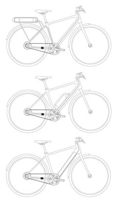
Rear and mid motor have different appreances, where the mid motor have motor in the middle of the bike and rear motor in the rear wheel of the bike. Even the LCD display and the display element may have a different appearance. Polygon pedelec are equipped with parts that work together to make the pedelec system powerful and natural. The dB level perceived by the driver is less than 70dB. The permissible overall weight for Polygon pedelec is 125 kg / 275 lbs.
